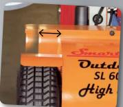
The lift has 100 mm sideshift for accurate adjustment when fitting the window
